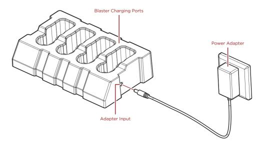
**NOTE:** Only use the provided adapter, using any other adapter may damage the equipment.
