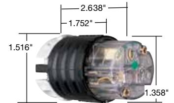
Dimensions for 15 & 20 Amp Connector
