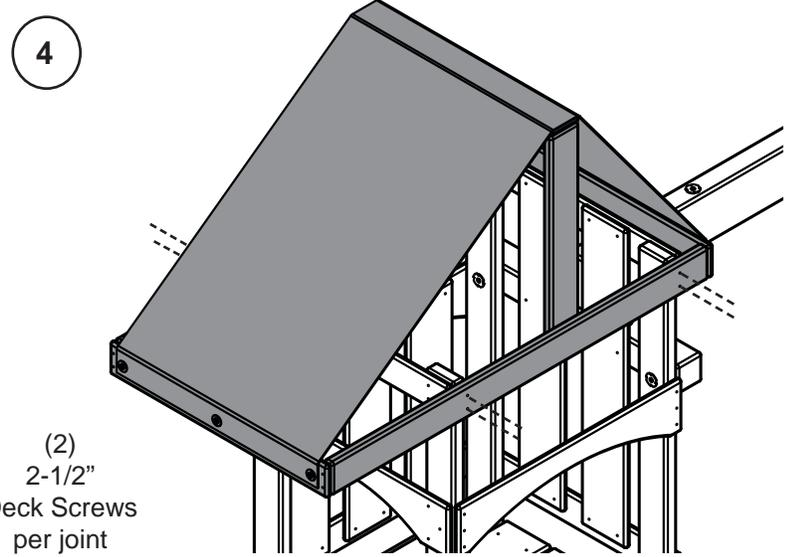
1. Assemble and install Roof as shown.
