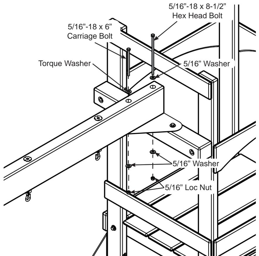
1. Attach Swing Beam to tower as shown.
