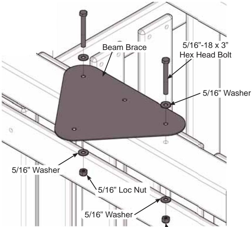
NOTE: Ensure two to three threads are exposed past Lock Nut.
