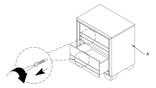
2 Secure with handle screw and tighten them by screw driver. (NOT INCLUDED)
