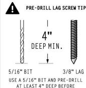
INSTALLING 3/8" LAG SCREWS
