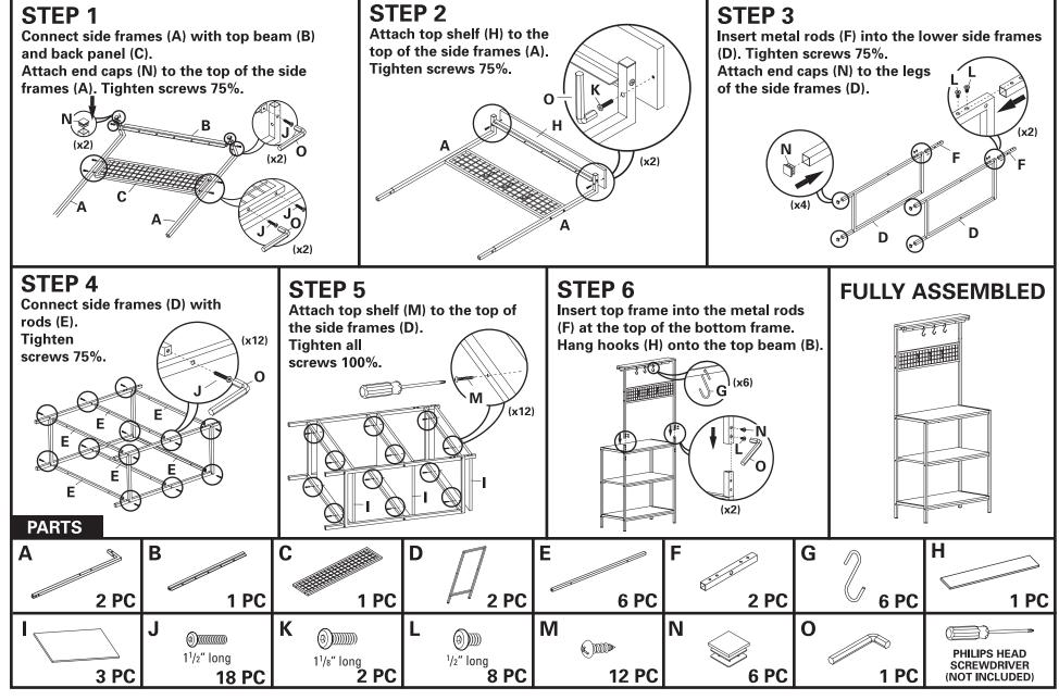
NOTE: PHILIPS HEAD SCREW DRIVER REQUIRED FOR ASSEMBLY (NOT INCLUDED) DO NOT TIGHTEN SCREWS 100% UNTIL FULLY ASSEMBLED.
