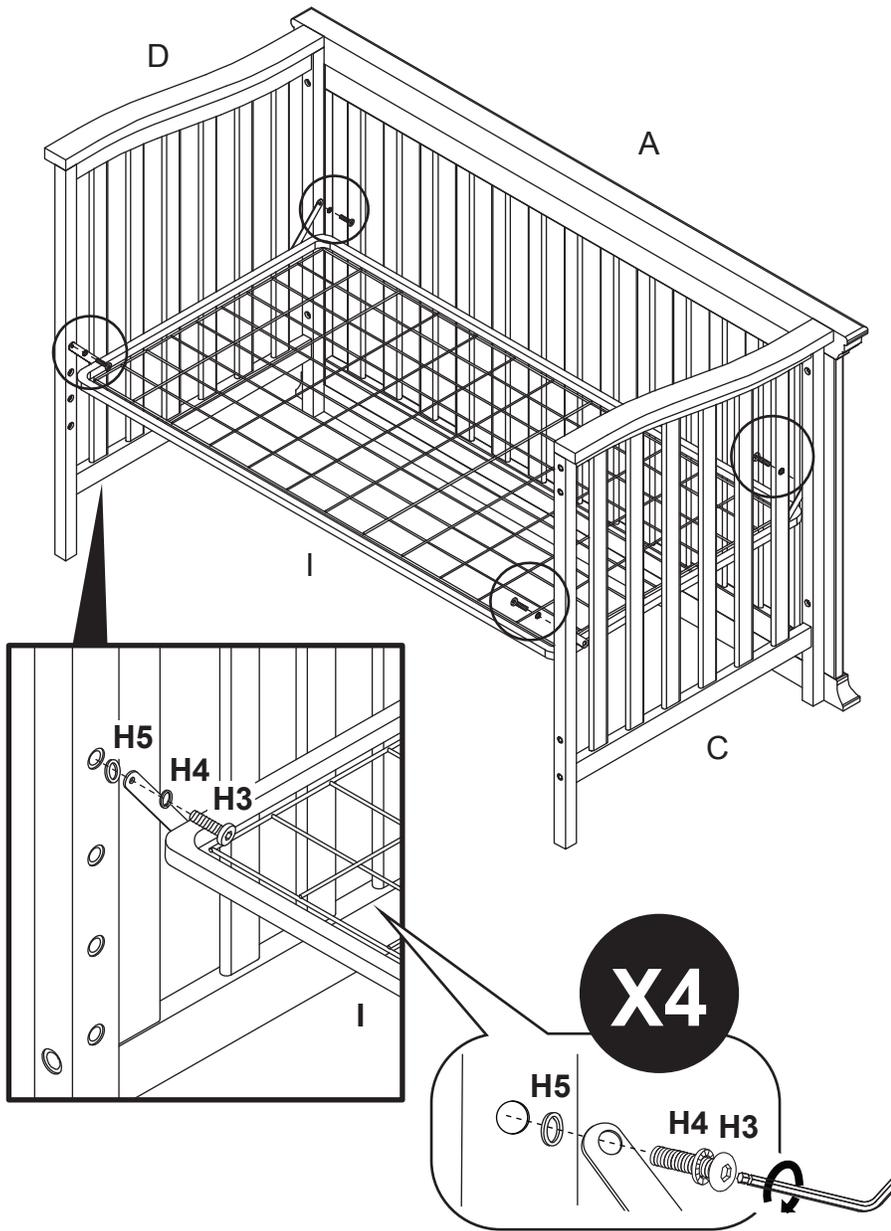
\* Make sure the mattress support III (I) is installed **FLAT SIDE UP**.
