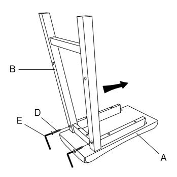
Insert Stretcher (C) into Leg Frame (B) and secure with JCBC/W (D) using Allen Key (E).
