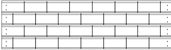
RP2 | UPPER ROOF PANEL - W2A03185 (x2) | 1 3/8"x12 3/4"x44 7/8" (35x324x1140)
