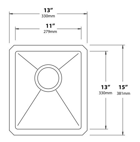
**NOTE:** Cutout template is provided as a guide **ONLY** and must be checked against actual sink to verify correct fit.
