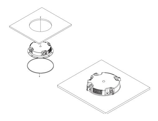
Step 4 - Reinstall magnetically retained grille.
