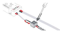
3. Use #1 Phillips to loosen the 4 terminal screws on 8MM-EZ Connector. Peel 1/2" of the adhesive protector from back of LED tape light, and scrape waterproof coating, insert into connector, evenly tighten screws. Insert wires from Wired Controller into terminals, Red wire to (+ or WW) side of tape, Black wire to (- or CW) side of tape; tighten screws.
