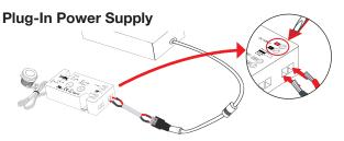
Cut a length of connection wire to run from Power Supply to Wired Controller. Strip 1/4" insulation from both ends of wire, twist each wire, and fold stripped wires in half. Use Female Barrel Connector (T-FBC) to run wire from Plug-in Power Supply. Red wire to (V+) terminal and Black wire to (V-) terminal on the wired controller.
