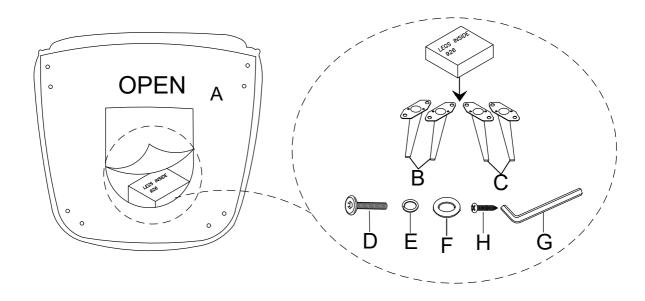
Attach the Leg (B) and the Leg (C) to the Chair (A) using Bolt (D), Spring Washer (E), and Flat Washer (F) with the Allen Key (G). Then, secure the Leg (B & C) to the Chair (A) using Screw (J) with a Phillips head screwdriver (not provided).
