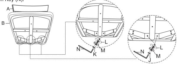
Keep the Backrest (A) and Cushion Seat (B) inverting on a stable raised surface. Attach the Swivel Plate located on the Apron with Swivel Plate (E) to the Cushion Seat (B) using JCBC Screw (I), Flat Washer (L) with Allen Key (N). Turn the Chair right side up.
