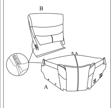
Step 2: Attach the RSF backrest (C) to the seat (A).
