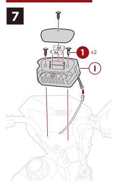
Use a screwdriver to open the compartment on the part I dashboard. Insert 2 AA batteries into the designated slots. Join the connector on the dashboard to the corresponding connector leading from the front frame.
