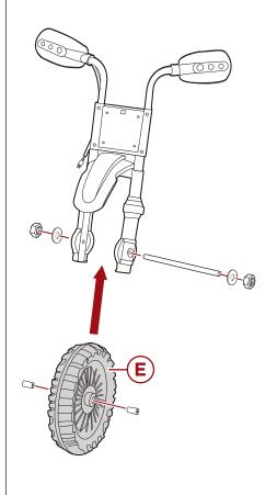
Remove the nuts, washers, spacers, and front axle from the part A handlebars.
