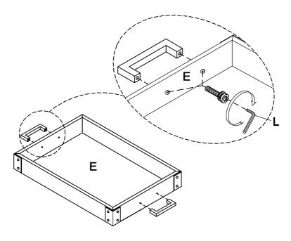
8 Attach the Top Tray (E) to the assembled cart.
