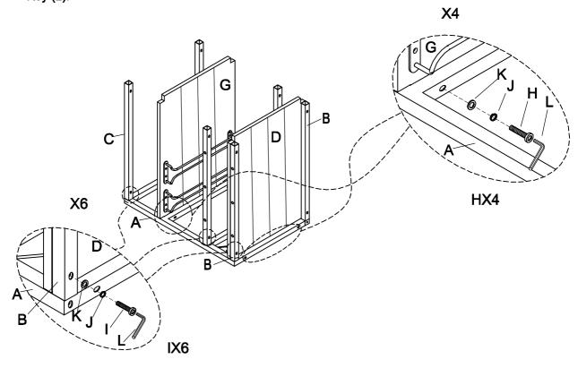
Attach the Side Frame (A) to the Lower Iron Stretcher (B) and Top Iron Stretcher (C) with Bottom Panel (D), Top Iron Stretcher (C) and Shelf (G)by using Flat Washer (K), Lock Washer (J) and Bolt-Small (I) with Allen Key (L) and Flat Washer (K), Lock Washer (J) and Bolt-Large (H) with Allen Key (L) as below showing.
