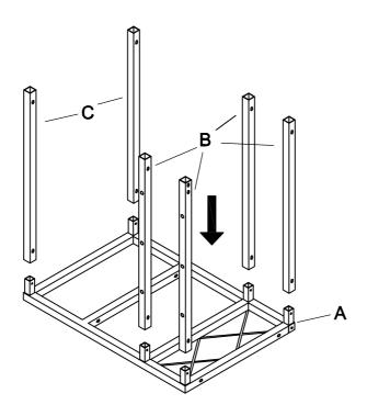
Attach the bottom Panel (D) and Shelf (G) to the Side Frame (A) by using Flat Washer (K), Lock Washer (J) and Bolt-Large (H) with Allen Key (L), and then Fix the Lower Iron Stretcher (B) and Top Iron Stretcher (C), by using Flat Washer (K), Lock Washer (J) and Bolt-Small (I) with Allen Key (L).
