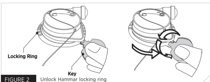
4. Turn the black locking ring counter clockwise and lift off the yellow cap. (Fig 3).
