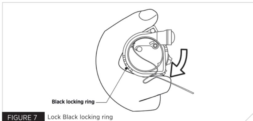
9. Check that the single point status indicator on the cap is green; that the pull to inflate lanyard is present; and that the locking ring is locked. Turn the inflation chamber and cover right-side out, returning to normal state.
