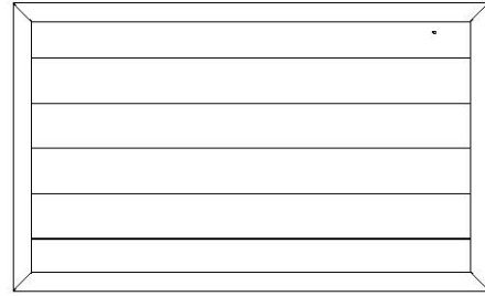
WP2 | PANNEAU MURAL - W2A02841 (x1) | 1 po x 20 3/8 po x 37 3/4 po (24 x 517 x 858)
