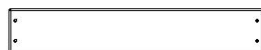
M9 | PLANCHE DE SOL - W4L13306 (x10) | 5/8 po x 3 3/8 po x 19 7/8 po (16 x 86 x 504)
