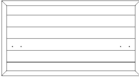
WP1 | PANNEAU MURAL - W2A02840 (x1) | 1 po x 20 3/8 po x 37 3/4 po (24 x 517 x 956)
