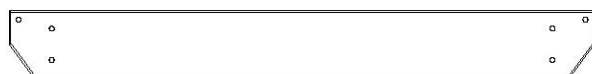
K14 | RAIL MURAL ANGULAIRE - W4L13194 (x1) | 5/8 po x 5 1/4 po x 45 3/4 po (16 x 134 x 1162)
