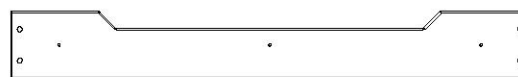
K10 | RAIL MURAL - W4L13174 (x1) | 5/8 po x 5 1/4 po x 40 1/2 po (16 x 134 x 1030)
