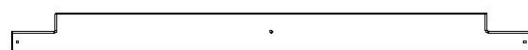
M16 | PLANCHE DE SOL - W4L13307 (x1) | 5/8 po x 3 1/8 po x 40 5/8 po (16 x 78 x 1031)
