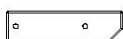
J3 | SUPPORT DE BANC - W4L13196 (x2) | 1 po x 2 3/8 po x 9 po (24 x 60 x 230)
