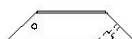
J4 | CALE ANGULAIRE - W4L13197 (x2) | 1 po x 2 3/8 po x 10 po (24 x 60 x 254)
