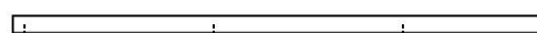
T5 | PLANCHE DE SUPPORT - W4L13313 (x1) | 1 po x 1 3/8 po x 37 5/8 po (24 x 34 x 956)
