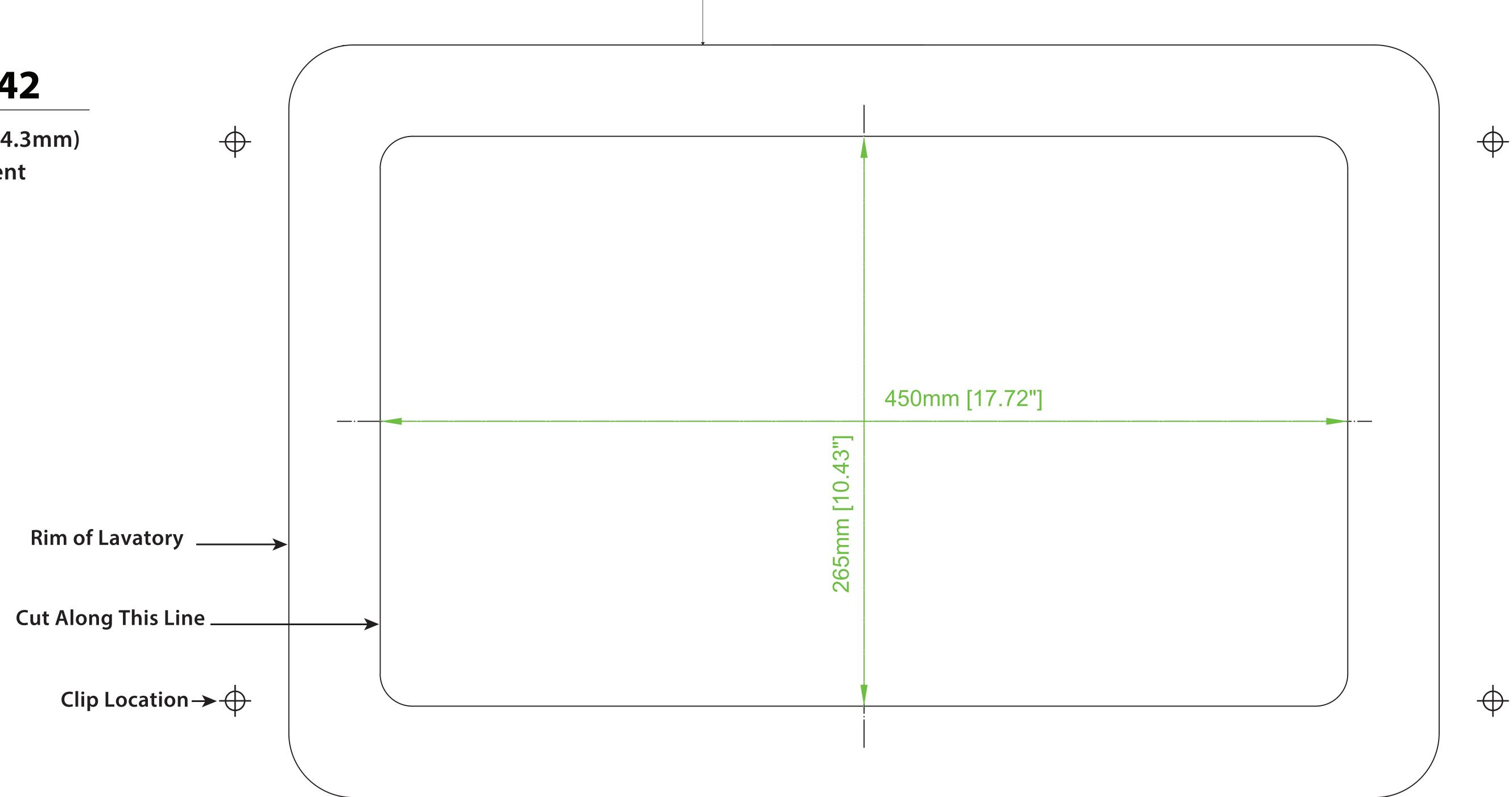
NOTE: When plotting template full size: Make sure horizontal and vertical dimensions match the dimensions labeled in the template
