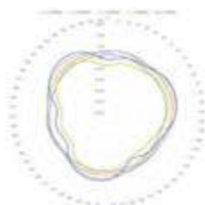
Azimuth Patterns, 2300 MHz-2700 MHz
