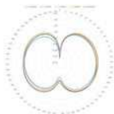
Elevation Patterns, 698 MHz-806 MHz
