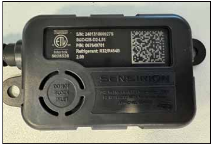
FIGURE 11. Example of Clear, Unobstructed Sensor Inlet
