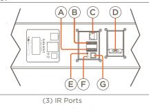
Uses 6-pin IR Connectors to send IR signals to control devices with an IR input or IR receiver via an IR flasher (5V tolerant only). See the Savant® IP Audio Products with Integrated Host Deployment Guide for important precautions regarding IR functionality before making any connections.
