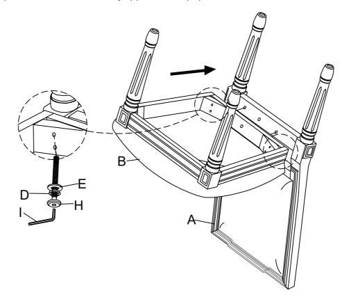
Finally, assemble the last Bolt (F) to Seat (B) and Chair Back (A) with Lock Washer
