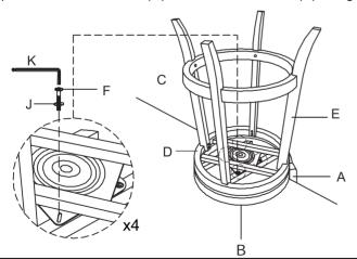
Stand chair up on an even surface and check that it is balanced. If there is a slight wobble, apply downward pressure in the corner where a leg is uneven. Keeping pressure in that corner, tighten all bolts. If balanced, apply downward pressure evenly in the center and tighten all bolts. Do not over-tighten beyond hole depth.
