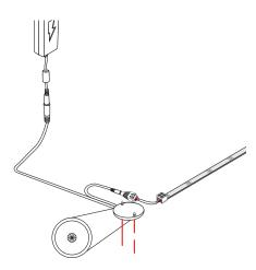
**1.** Insert Male Plug on Power Supply into Female Plug on Motion Sensor. Insert Male Plug on Motion Sensor into Female Connector on lights.
