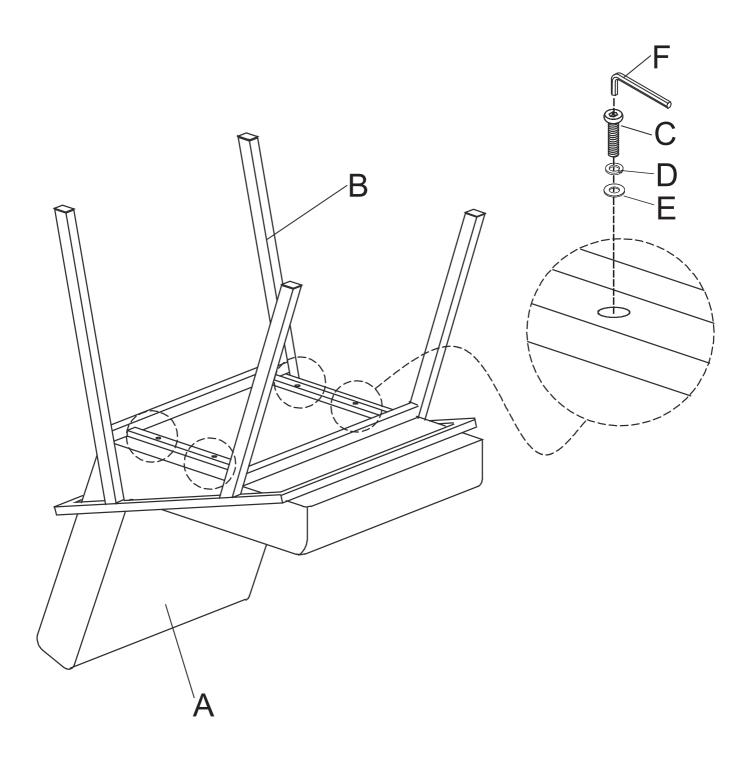
Take the Allen Wrench and turn the bolts until the legs are secured. DO NOT TIGHTEN THE BOLTS COMPLETELY. Stop when you feel you are adding force to tighten the bolt.
