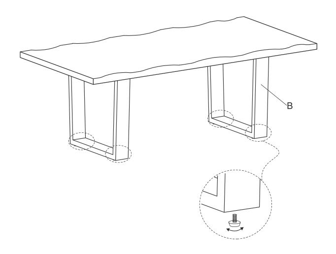
Turn left or turn right to adjust the leveler until the table is stabilized.
