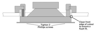
A snug fit is all that is necessary to assure proper performance.
