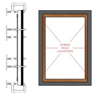
Mounting screw holes are located in the gasket channel behind the gasket.
