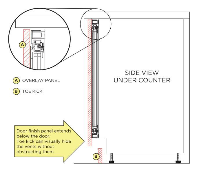
The XOU24 GOA series is 32 1/4" Tall. The standard US undercounter refrigerator is 34" Tall. Allow the additional panel length to extend as an apron below the door.
