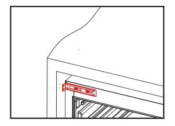
With the door open, using the screws provided connect the tie in bracket in the upper corner of the wine cooler opposite the hinge then screw the flange of the bracket to the cabinet.
