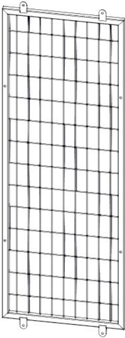
MP01 PANNEAU MÉTALLIQUE - A4M02614 (x6) 1 1/16"X20 1/2"X58 9/16" (27.4x520x1488)
