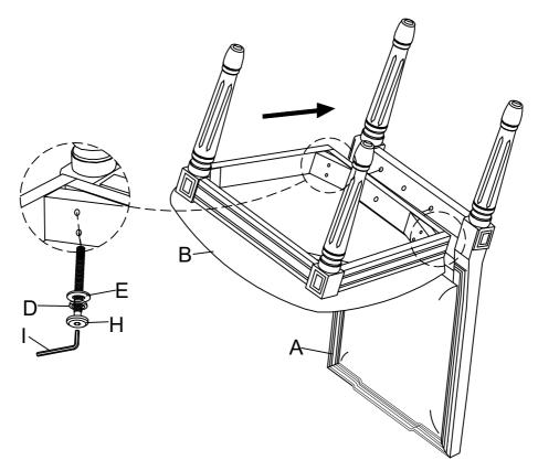
Finally, assemble the last Bolt (F) to Seat (B) and Chair Back (A) with Lock Washer (D) & Flat Washer (E) by Allen Key (I).
