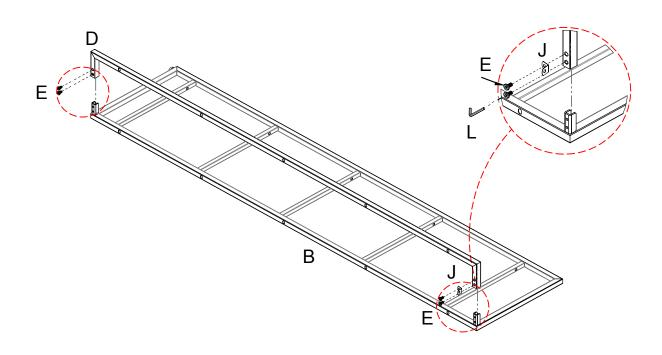
Attach Mounting Plate (J) to the Back Frame (D) and Side Frame - LSF (C) with Bolt (E) and Allen Wrench (L), making sure the Mounting Plate (J) extend DOWNWARD as shown.
