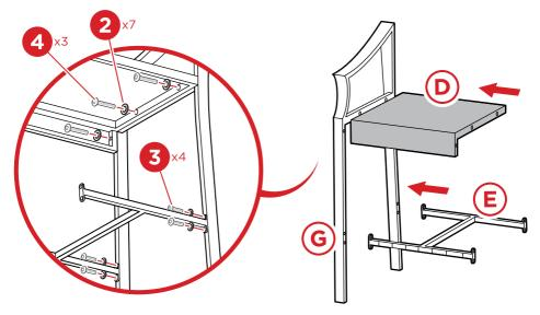
2 Locate and attach one part H left chair leg to the part D seat frame with three part 4 screws and three part 2 washers.
