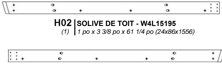
H09 | SOLIVE DE TOIT - W4L15213 (1) | 1 po x 3 3/8 po x 61 1/4 po (24x86x1556)
