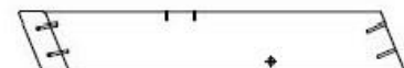
E13 | CHEVRON - W4L15219 (2) | 1\frac{3}{8} po x 3\frac{3}{8} po x 21\frac{15}{16} po (36x86x557)
