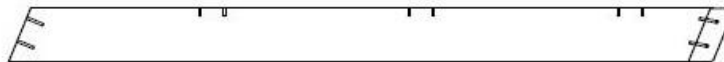
E06 | CHEVRON - W4L15208 (2) | 1\frac{3}{8} po x 3\frac{3}{8} po x 45\frac{7}{16} po (36x86x1155)
