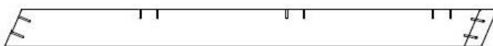
E09 | CHEVRON - W4L15211 (2) | 1\frac{3}{8} po x 3\frac{3}{8} po x 44\frac{1}{16} po (36x86x1119)
