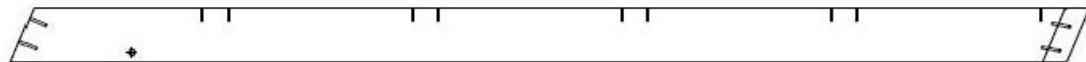
E08 | CHEVRON - W4L15210 (2) | 1\frac{3}{8} po x 3\frac{3}{8} po x 67\frac{5}{8} po (36x86x1717)
