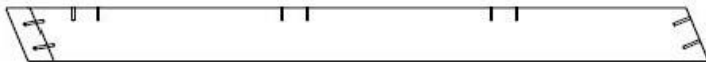
E03 | CHEVRON - W4L15199 (2) | 1\frac{3}{8} po x 3\frac{3}{8} po x 44\frac{1}{16} po (36x86x1119)
