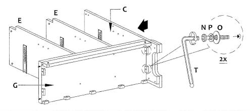
Place Back Top Rail (F) to Center Panel (E) and tighten it with Flat Washer (O), Spring Washer (P) and JCBC Bolt (N). Insert Minifix Housing (L) to Side Panel (Left)(C) and follow the arrow to lock it.
