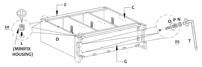
Turn the Front Frame (B) upside down and place it on a piece of cloth to prevent from scratching. Gently insert the semi asembled Server to the Front Frame (B). Insert Minifix Housing (L) and follow the arrow to lock it.
