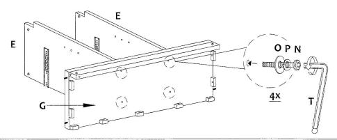
Gently insert Side Panel (Left) (C) to the Bottom Panel (G) and secure it with Flat Washer (O), Spring Washer (P) and JCBC Bolt (N) and tighten with Allen Key (T).
