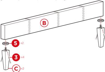
Screw two part C bed legs and two part 5 plastic spacers into the part A headboard. Secure the bed legs with four part 3 screws, two screws per leg.
