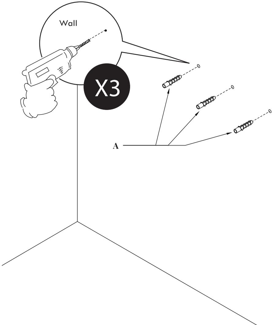
Use power drill (not provided) to open three holes at the marked areas. Insert the Plastic Wedge **A** into the holes with a hammer (not provided).
