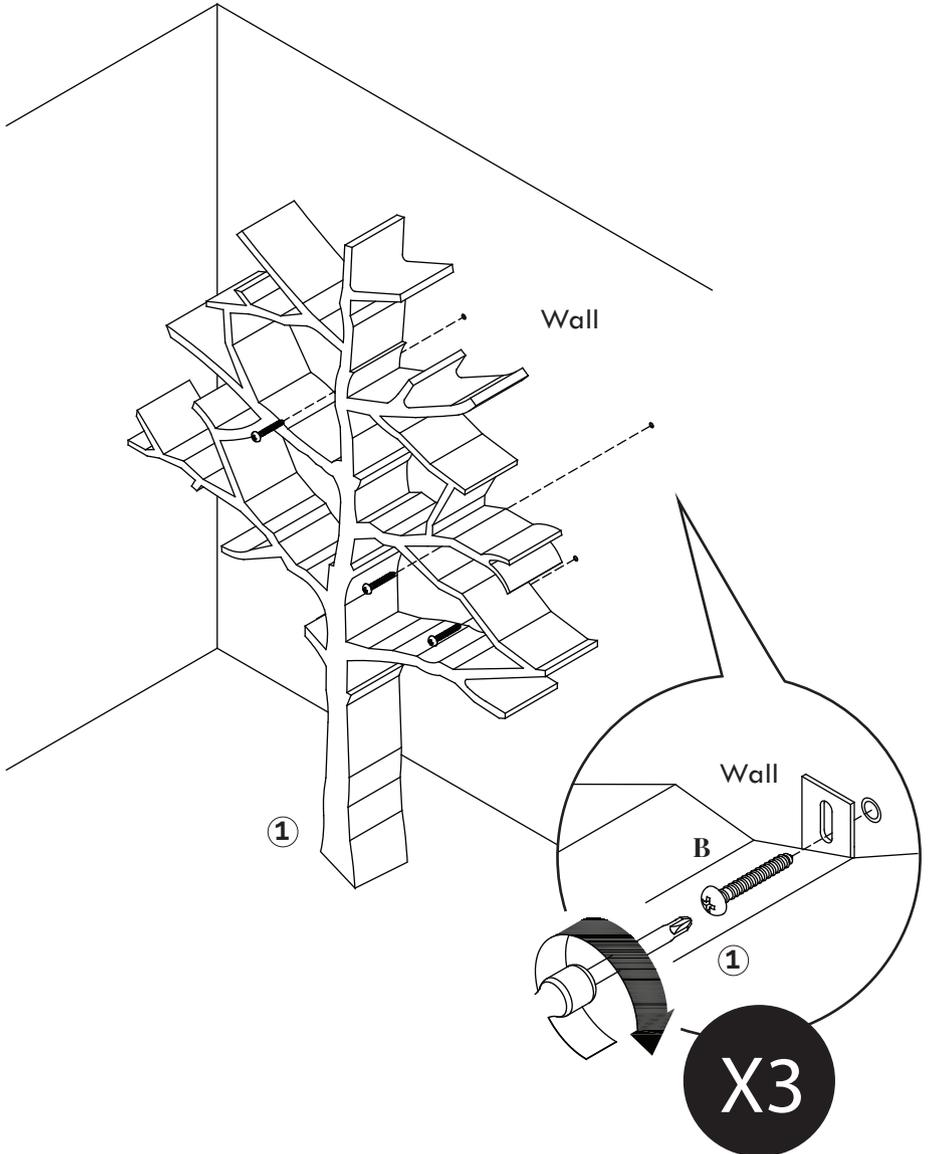
Position the Tree Bookcase ① back on the wall again and secure the metal plates with Screw **B** and a Phillips Head screwdriver (not provided).
