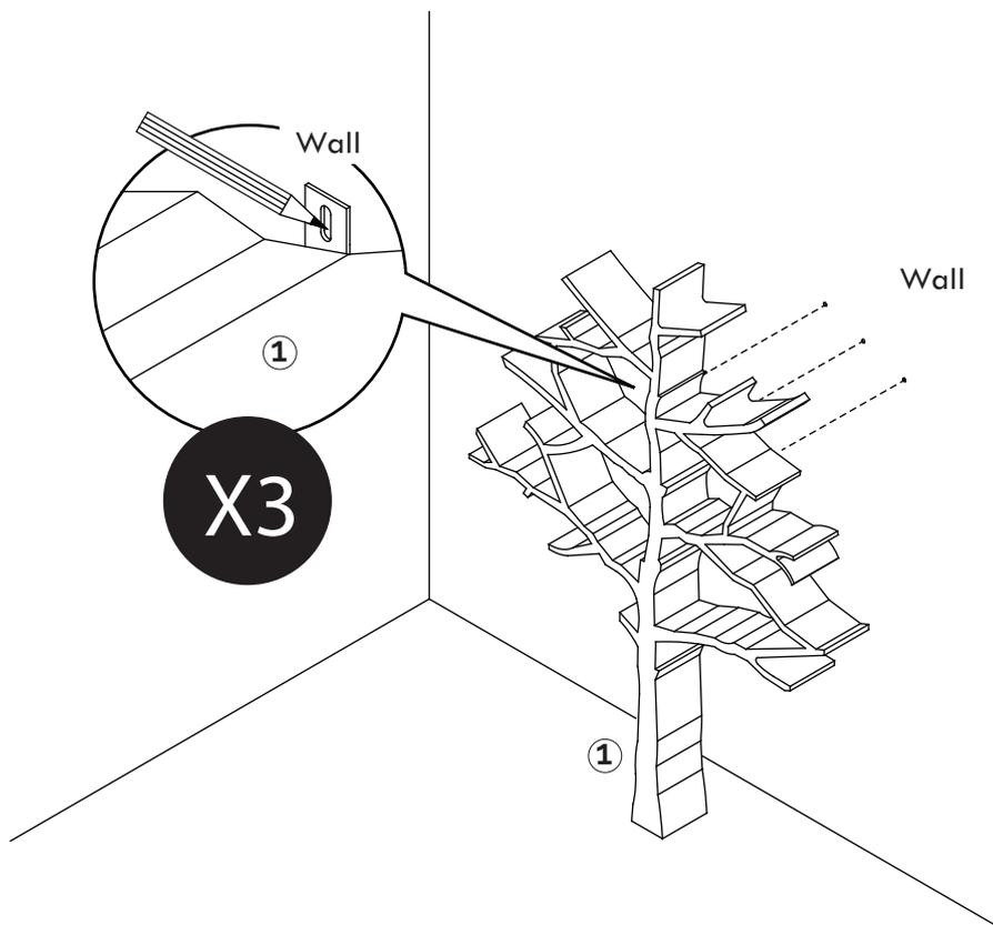
Position the Tree Bookcase ① on the wall. Make sure the installation area is clean. Mark the wall where the metal plates are located.
