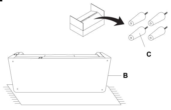
Tighten each Leg (C) in a clockwise direction.
