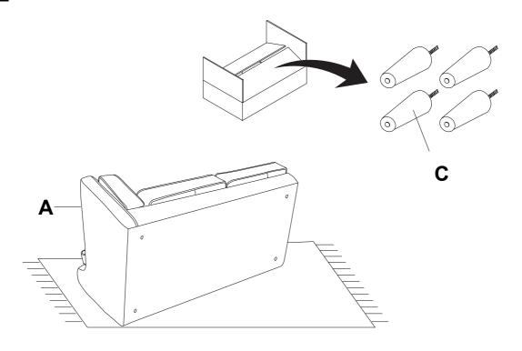
Tighten each Leg (C) in a clockwise direction.
