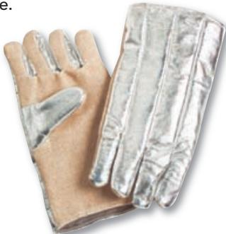
**234-AZ-Z** Combo glove. 35 oz. Zetex® glass on palm for short durations up to 1000°F. 25 oz. aluminized Zetex® for up to 2000°F radiant protection on back side. Moderate to poor abrasion resistance.
