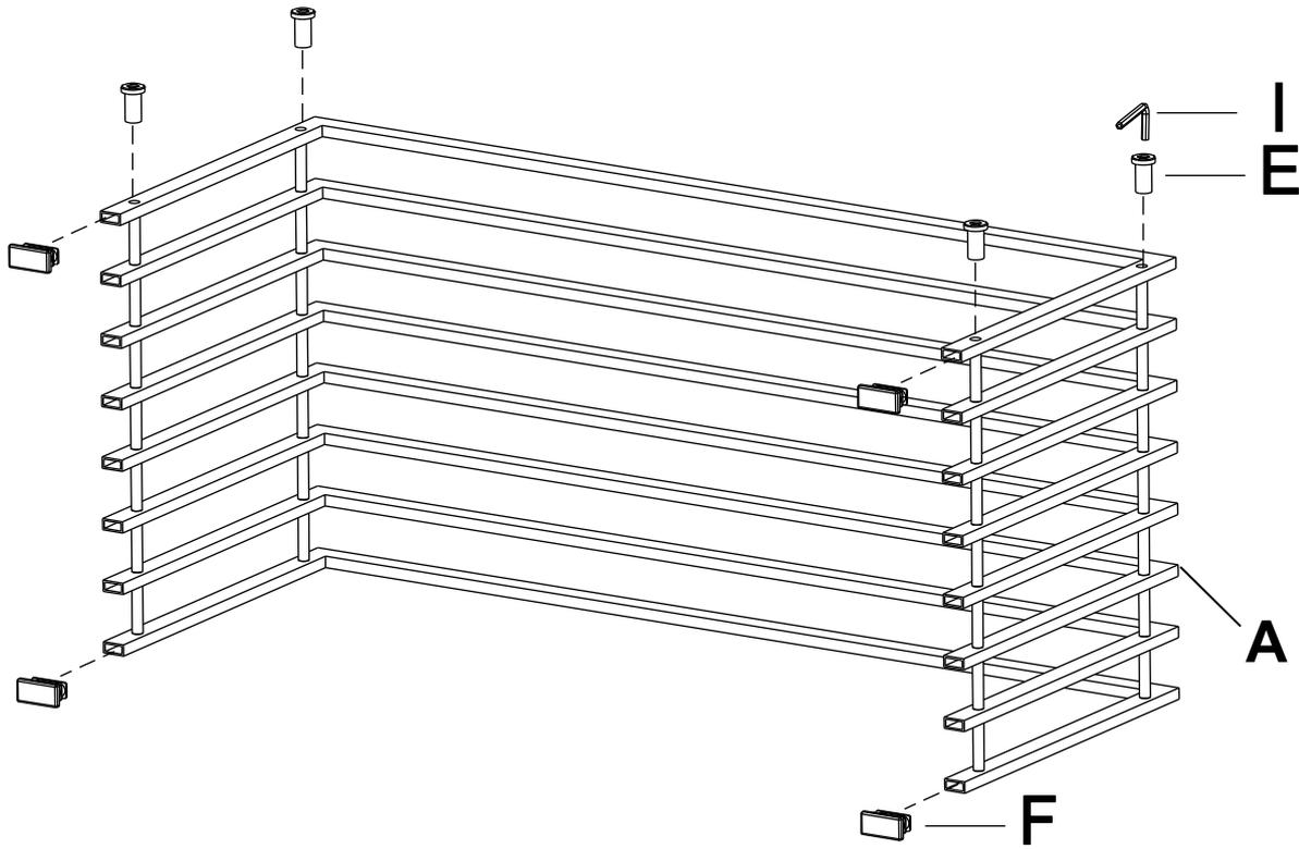
**4** Use two Allen Wrench (I) to tighten all bolts. Make sure all bolts are tightened, then cover the bolt head by Bolt Cover (G) as shown.
