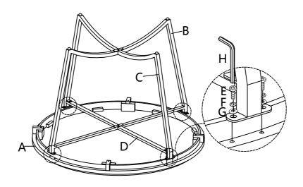
Adjust the pre-installed levelers at the bottom of Support Frame (B) and Side Frame (C) until the Dining Table is level with the ground.
