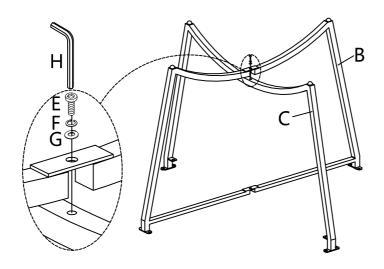
Stand the base frame up. Using Bolt (E), Spring Washer (F), Flat Washer (G) with Allen Key (H) to fix Rail (D) to Side Frame (C) and Support Frame (B).
