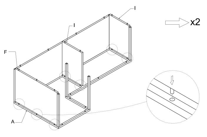
Attach the Shelf Board (E, G, H) to the Side Frame - Front (A).
