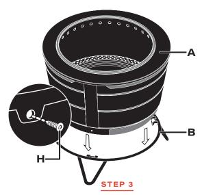
Place the Fire Pit (A) on top of the foot ring (B) ensuring the 3 tabs on the foot ring align with the 3 holes at the base of the Fire Pit and secure with 3 screws (H) using the supplied Hex Key.
