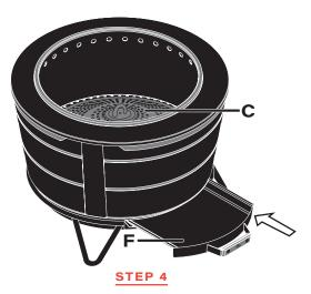
Replace the ash pan (F) and dome insert (C) back into the Fire Pit.
