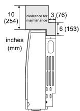
Clearances to access the furnace during servicing are 10 in. (254 mm) from the sides, 40 in. (1 m) from the front, and the area shown above the furnace in the figure to the left.
