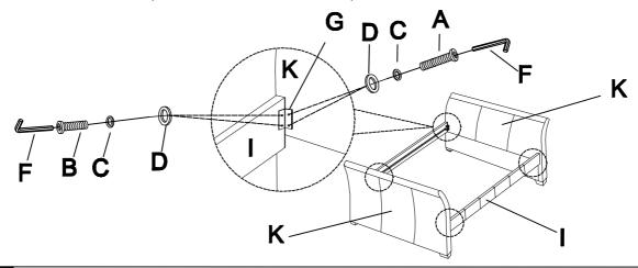
Attached Back Rest(H) to Left & Right Arm(K), and attached Bolt(A), Lock Washer(C), Flat Washer(D), turn the Allen Wrench(F) in Blot(A).
