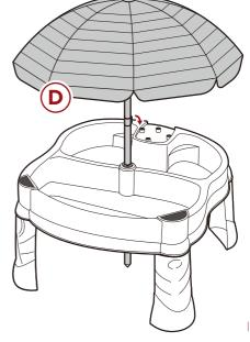
**NOTE:** Please add minimum insertion depth (2.5 in) of top section into the lower section.
