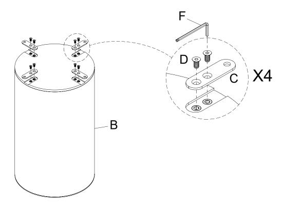
Attach the Column Base (B) to the Top Panel (A) using Bolt (E) through the Metal Bracket (C) with the Allen Key (F).
