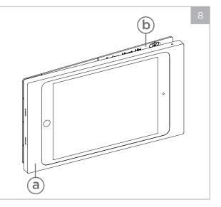
With the iPad home button facing left or right, the Surface Mount will attach to the (b) mounting bracket with internal magnets.
