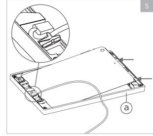
Plug in the provided IPORT USB-C cable directly into the iPad. Position the iPad Face down into the (a) bezel with the iPad cable on the left. Carefully wrap the iPad cable under the retention loop located on the (a) bezel. To lock the iPad in place, use a flat head screwdriver to deploy the second and third toggles located on th right side of the Surface Mount (a) bezel. The first top-right toggle is a power button extension.
