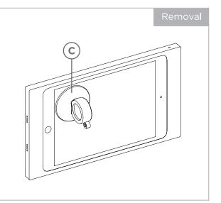
The (c) suction cup (provided) is used to remove the iPad and (a) bezel from the (b) mounting bracket. Once the (a) bezel is unlocked from the (b) mounting bracket, depress the (c) suction cup on the corner of the iPad screen and carefully pull the iPad from the wall, while the other hand is supporting the opposite side of the (a) bezel.
