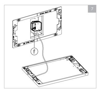
Connect the appropriate power source identified in the Power and Wiring Guide (found in (f) PoE splitter box). Place the PoE splitter into the single gang box located in the wall.
