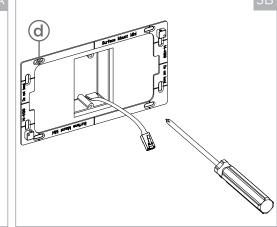
Using the recommended screwdriver and (d) mounting screws, install the first screw in the upper left-hand corner.
