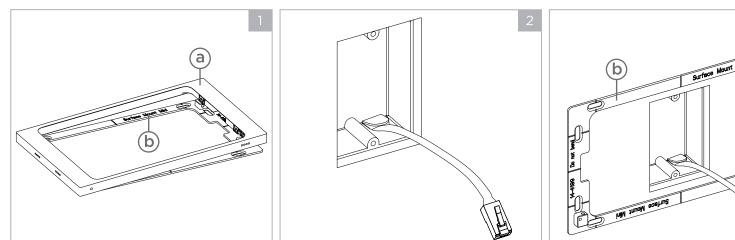
When removing the Surface Mount (a) bezel from its box. the bezel will be attached to the (b) mounting bracket. To decouple the (a) bezel from the (b) mounting bracket, place the (a) bezel face up on a flat and smooth surface. With one hand, hold the (b) mounting bracket in place. With your opposite hand, lift the right edge of the (a) bezel and then the left to decouple the magnets. This will help avoid bending of the metal, and prevent any damages to the (a) bezel or (b) mounting bracket.
