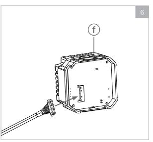
Connect the USB-C to Molex cable into the (f) PoE Adapter shown.
