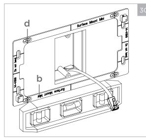
Level the (b) mounting bracket over wiring location and fasten (b) bracket with the remaining (d) screws. Lining up the (d) mounting screws with the engraved center lines provided on the (b) bracket will allow you optimal adjustability. The (b) mounting bracket is now in place.
