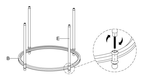
2 Assemble Bottom Frame (D) with Support Post (E) using Leg (F) as below shown.
