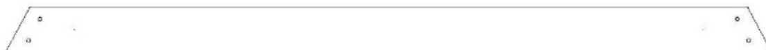
G08 | PLANCHE DE SOL - W4L15894 (1) | 1 po x 5 1/4 po x 86 3/4 po (24 x 134 x 2 202)
