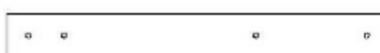
H18 | RAIL MURAL DU PAVILLON - W4L04616 (1) 1 po x 3 3/8 po x 29 7/8 po (24 x 86 x 758)
